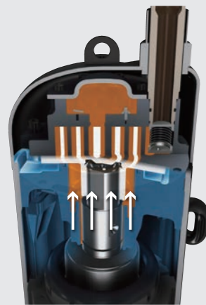
The force pressing the orbiting scroll decreases during low-load operation.
